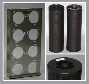
Cylindrical sorbent canisters attach to an easy-slide holding frame for installation into a Camsorb GlidePack side-access housing (top). Standard plastic sorbent canisters (middle right) mount to the frame with a unique bayonet bolt mount. A tool is provided that tightens the cylinder to the frame and ensues an air tight seal (see Product Sheet 2112 for cylinder information). (Housing above shown with optional metal cylinders and MERV 7 prefilter).
